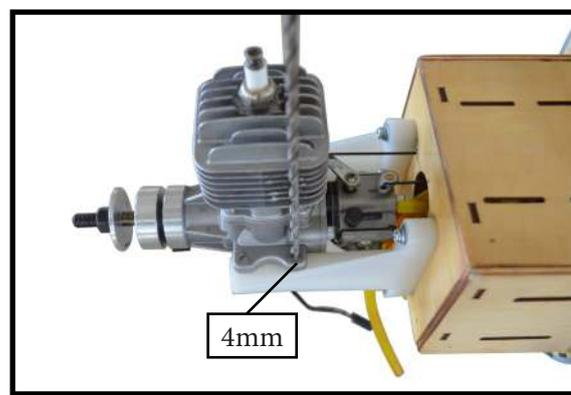
Use a drill to drill the four holes in the engine mount rails.
