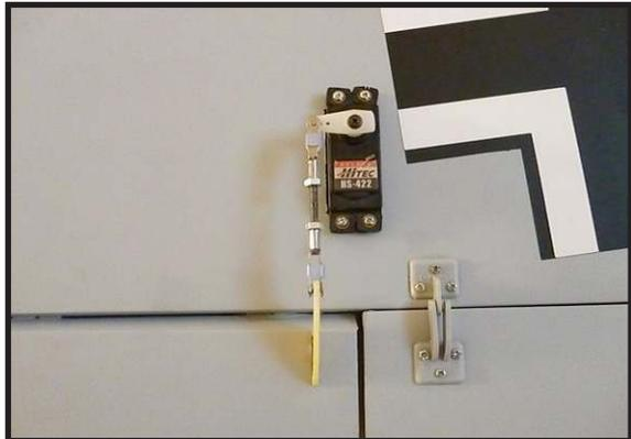
**INSTALLING THE FLAP SERVO.**
