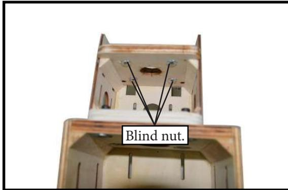
Attach the motor to the front of the electric motor box using four 4mm blind nut, four M4x20mm hex head bolts to secure the motor. Please see picture shown.
