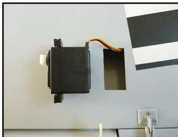
Set the aileron servo in place and use a Phillips screw driver to install it with four wood screws.
