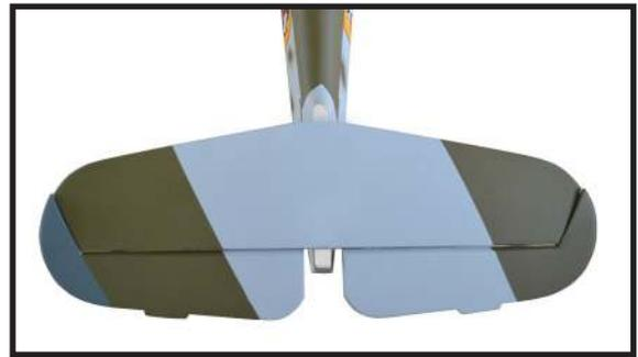
With the stabilizer held firmly in place, use a pen and draw lines onto the stabilizer where it and the fuselage sides meet. Do this on both the right and left sides and top and bottom of the stabilizer.
