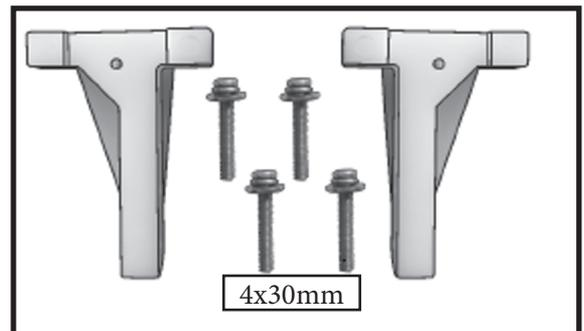
Use four 4x30mm head bolts and four 4mm washers to attach the engine mount rails to the firewall. Tighten the screws . Make sure to use threadlock on the screws to help prevent them from vibrating loose.
