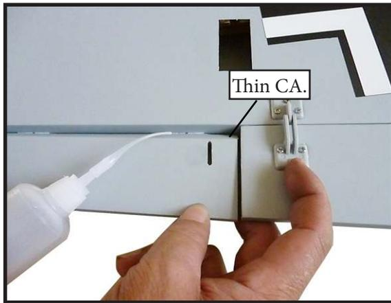
Turn the wing panel over and deflect the aileron in the opposite direction from the opposite side. Apply thin C/A glue to each hinge, making sure that the C/A penetrates into both the aileron and wing panel.
