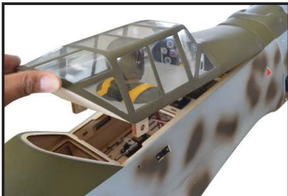
Position the pilot figure on the canopy floor as shown. Use epoxy to glue the base of the pilot figure to the cockpit floor, please see pictures as shown.
