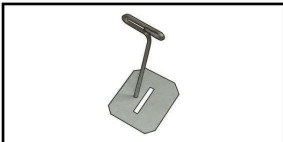
Remove each hinge from the wing panel and aileron and place a T-pin in the center of each hinge. Slide each hinge into the wing panel until the T-pin is snug against the wing panel. This will help ensure an equal amount of hinge is on either side of the hinge line when the aileron is mounted to the aileron.
