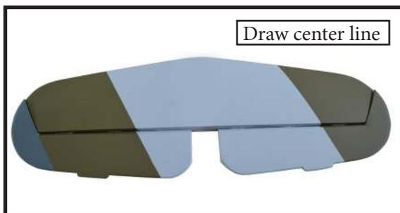
Using a modeling knife, carefully remove the covering at mounting slot of horizontal stabilizer ( both side of fuselage).
