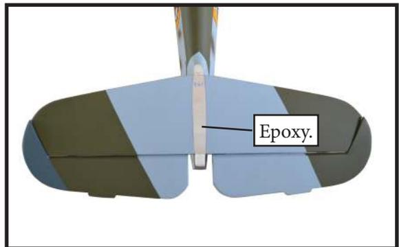
Slide the vertical stabilizer back in place. Using a triangle, check to ensure that the vertical stabilizer is aligned 90° to the horizontal stabilizer.
