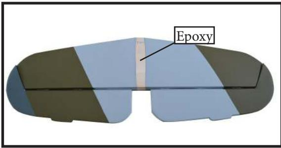
When you are sure that everything is aligned correctly, mix up a generous amount of 30 Minute Epoxy. Apply a thin layer to the top and bottom of the stabilizer mounting area and to the stabilizer mounting platform sides in the fuselage. Slide the stabilizer in place and realign. Double check all of your measurements once more before the epoxy cures. Hold the stabilizer in place with T-pins or masking tape and remove any excess epoxy using a paper towel and rubbing alcohol.
