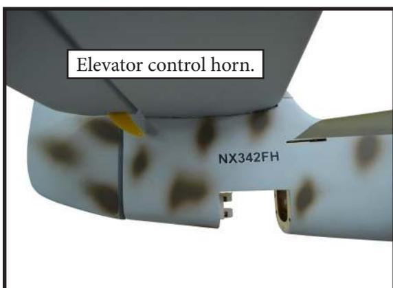
Thread one clevis and M2 lock nut on to each elevator control rod. Thread the horns on until they are flush with the ends of the control rods.
