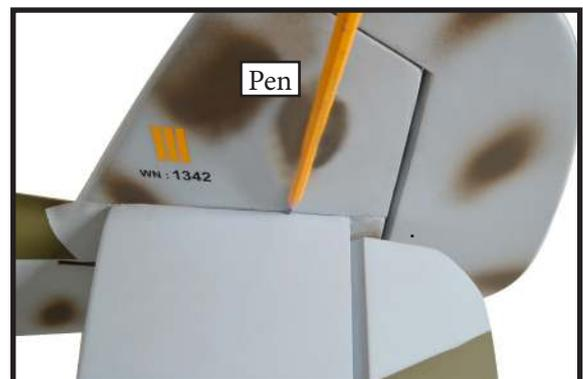
Remove the stabilizer. Using the lines you just drew as a guide, carefully remove the covering from between them using a modeling knife.
