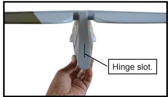
While holding the vertical stabilizer firmly in place, use a pen and draw a line on each side of the vertical stabilizer where it meets the top of the fuselage.
