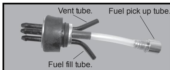
Carefully bend the second nylon tube up at a 45° angle. This tube is the vent tube.
