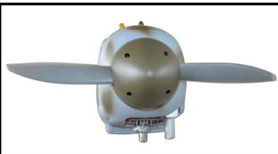
⚠ The propeller should not touch any part of the spinner cone. If it does, use a sharp modeling knife and carefully trim away the spinner cone where the propeller comes in contact with it.
