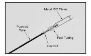
Use a felt tip pen to mark the wire where it crosses the hole. Use a pair of pliers to put a shrp 90-degree bend in the wire at the mark.
