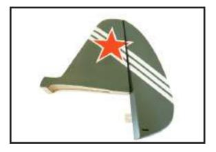
1) Using a modeling knife, remove the covering from over the precut hinge slot cut into the lower rear portion of the fuselage. This slot accepts the lower rudder hinge.
