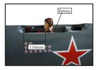
4) Position the canopy onto the fuselage. Trace around the canopy and onto the fuselage using a felt-tipped pen. Carefully cut and remove covering material from the fuselage where the canopy makes contact, exposing the bare wood. Then permanently glue the canopy in place with epoxy glue or special "canopy glue".
