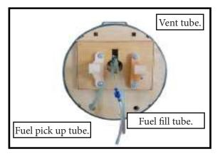
8) Connect the lines from the tank to the engine and muffler. The vent line will connect to the muffler and the line from the clunk to the carburetor.
