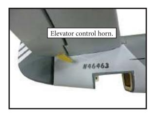
3) Thread one clevis and M2 lock nut on to each elevator control rod. Thread the horns on until they are flush with the ends of the control rods.
