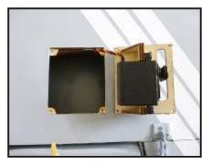
9) Set the aileron hatch in place and use a Phillips screw driver to install it with four wood screws.
