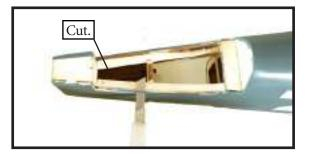
3) Slide the stabilizer into place in the precut slot in the rear of the fuselage. The stabilizer should be pushed firmly against the front of the slot.
