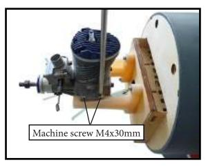
4) On the fire wall has the location for the throttle pusshrod tube (pre-drill).
