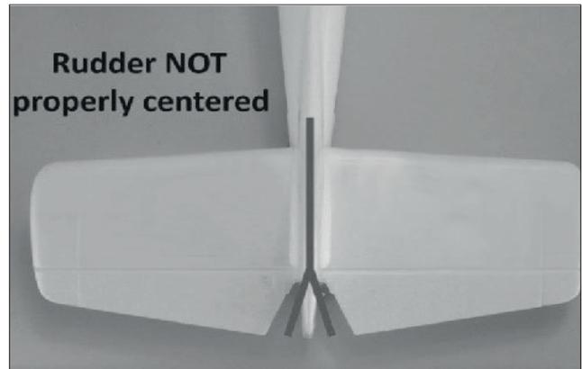
Observe the rudder to ensure it is properly centered as shown above.
