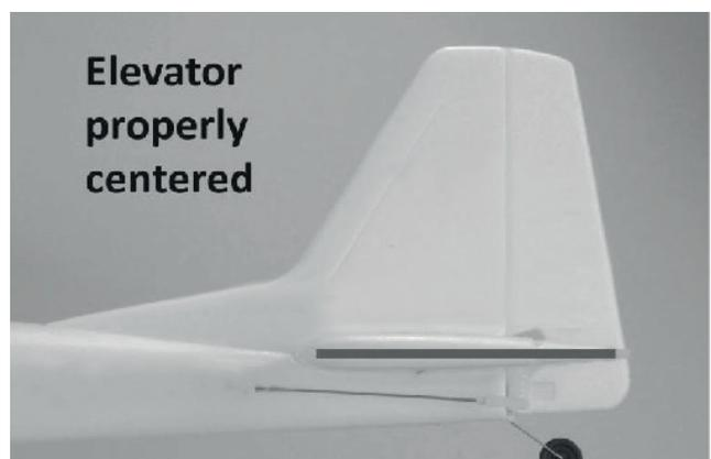
Then observe the elevator to ensure it is properly centered as shown above.
