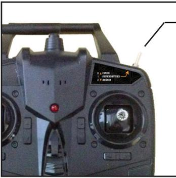
To enable easy flying, the Easy Trainer is supplied with a pre-installed gyro. To turn on the gyro, slide the stick to the "Anfänger" (Beginner) position. To turn the gyro off, slide the stick toward the "Experte" (Expert) position. The center position allows a weaker gyroscopic effect.
