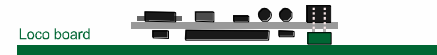
21-pin decoder plugged into loco board, i.e. TRIX Plugged in right side up, pins of the loco board penetrate through the decoder board into the socket.
